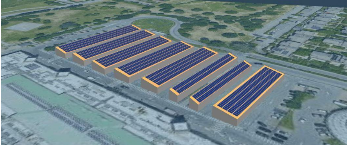
Collective Self-Consumption Project: PV system on parking area shelters. Via Larga Shopping Center, Bologna
